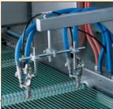
Spray-unit with mechanical height adjustment
